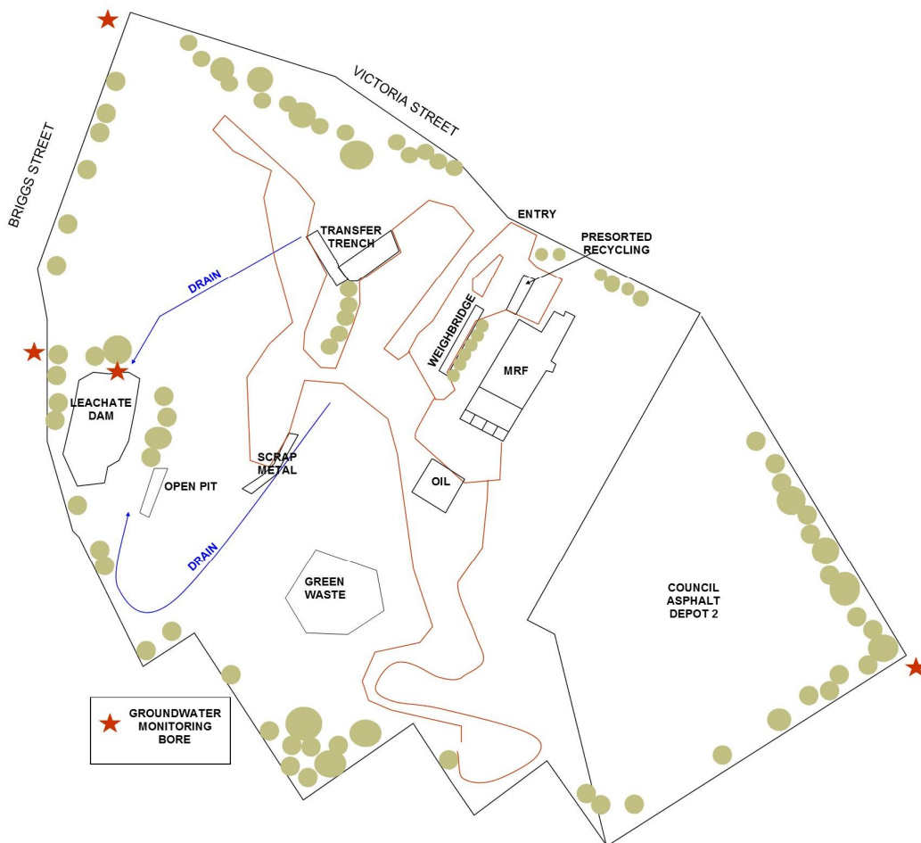
Image 2: Site Plan indicating drainage and leachate dam.
