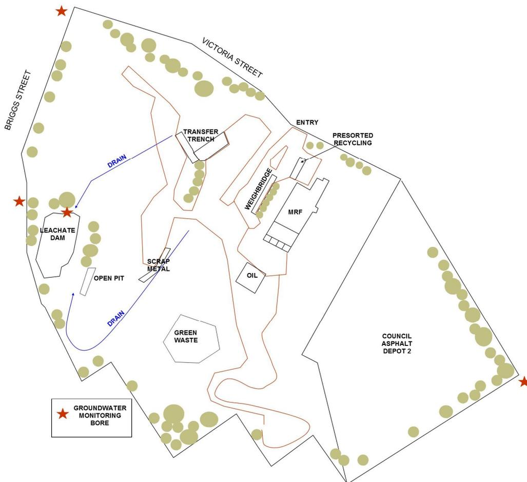
Image 2: Site Plan indicating drainage and leachate dam.
